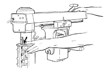
2. Loosen (2) %-20 Gib set screws on the left side at the rear of the column support.
